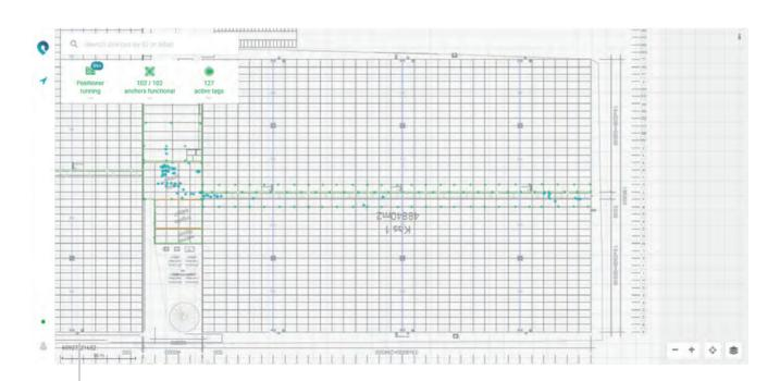
The Pozyx team provided assistance to ensure that every greenhouse was fully covered. A single 48840 m<sup>2</sup> indoor greenhouse area was quipped with over a 100 Anchors. By daisy chaining multiple anchors, the total cabling needed was kept to a minimum.
