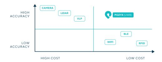
On the right side, you'll find all the radio-based technologies (generally cheaper), and on the left side, you'll find all the light-based technologies (typically more expensive). Likewise, you can see on the matrix that light-based technologies will generally be more accurate; this is because of standard physics principles.
